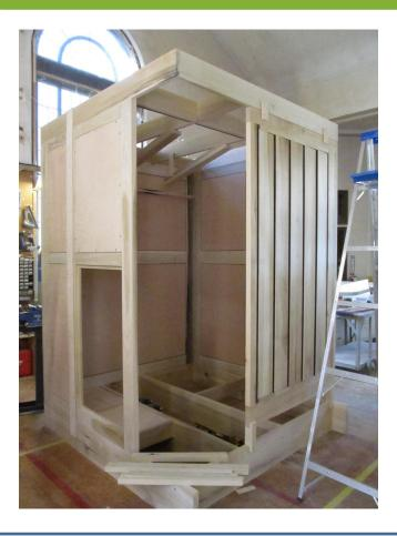
To the left is a photo of the "swell box" in the process of being assembled. It will house all but the largest 24 of the 402 pipes that will make up the new Swell division. Five of the seven louvers to control sound volume are in place in the closed position. The new stop rail is nearing completion. In October we will install that in the console and connect it to the organ's existing stops.
