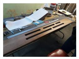
1. This is the new solid walnut stop rail, into which 68 new stop switches will be installed, replacing the original plywood one with 23 stops.
