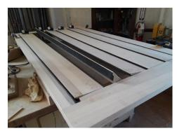
4. This is the larger of the two panels of louvers – commonly called swell shades. These are controlled by a pedal on the console, allowing the organist to infinitely vary the amount of sound coming through them.
