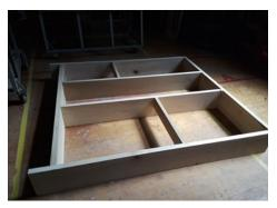
3. This is the Swell impost. It will attach behind the existing Great division (upper middle part of the organ). This is what supports the windchests on which all but 24 of the 402 pipes of the new Swell division will stand. It will also support walls on three sides and two panels of louvers in front.
